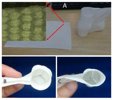
Fig. 1 Processing 2D, polycaprolactone (PCL) fabric (a) into three dimensional and functional heart valve including sinuses and leaflets, for native valve replacement (b&c). Red arrows indicate the close-up view of the fabric, the plot of the single thread is visualized
